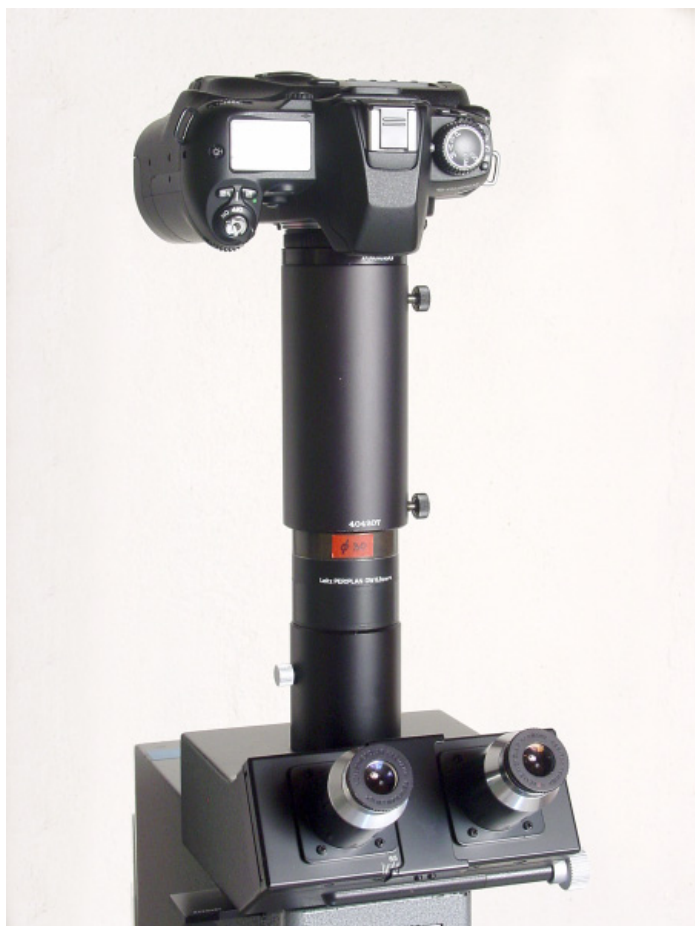
Figure 1. Microscope manufacturers typically offer their own SLR adapters. This one is made for Leica microscopes. A cylindrical sleeve connects the photo eyepiece (8x or 10x) to the camera lens (0.32x). As long as the eyepiece is of the type that matches the correction characteristics of the objectives, optimal optical performance and parfocality are assured.
