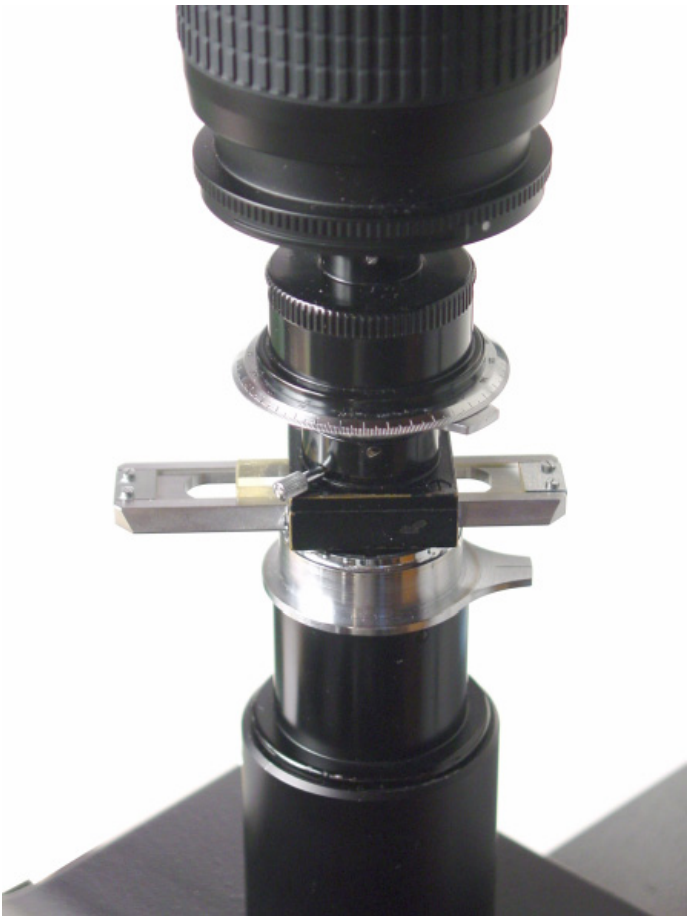
The Wright eyepiece with Johannsen quartz double wedge reveals the magnitude of the retardation (1500nm) and the positive sign of elongation (hyperbola shaped extinction band) of this Nylon fiber in one spectacular view (lower left of page). The use of a DSLR makes it possible to photograph and preserve the unique appearance of a circular field which is partially cut off at two diametrically opposed points by the frame of the wedge.
